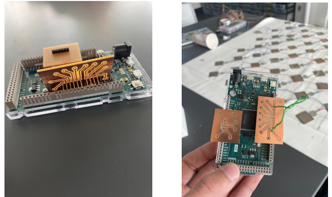
Figure 5. 3D printed circuit board serving as a featherboard connection between the sensor array and Arduino Due
